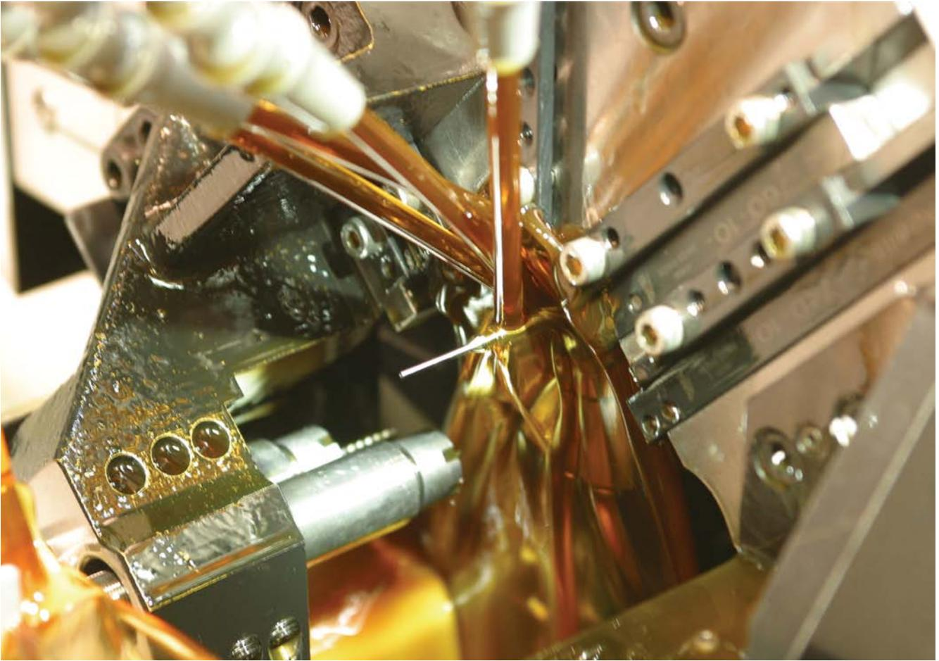
*Closeup view of a titanium phaco tip in production in a Citizen Cincom B12. The parts are flooded with American Research Products Amerilube 30, an ultra-low VOC cutting oil, which has increased tool life. The cutting oil meets SCAQMD "super compliant" specifications, which in most cases eliminates the need for record keeping.*
